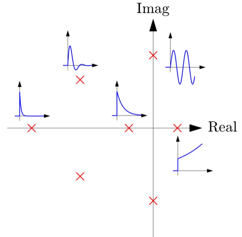
A system (open or closed) is BIBO-stable iff  $\text{Re}(p_i) < 0$ .
