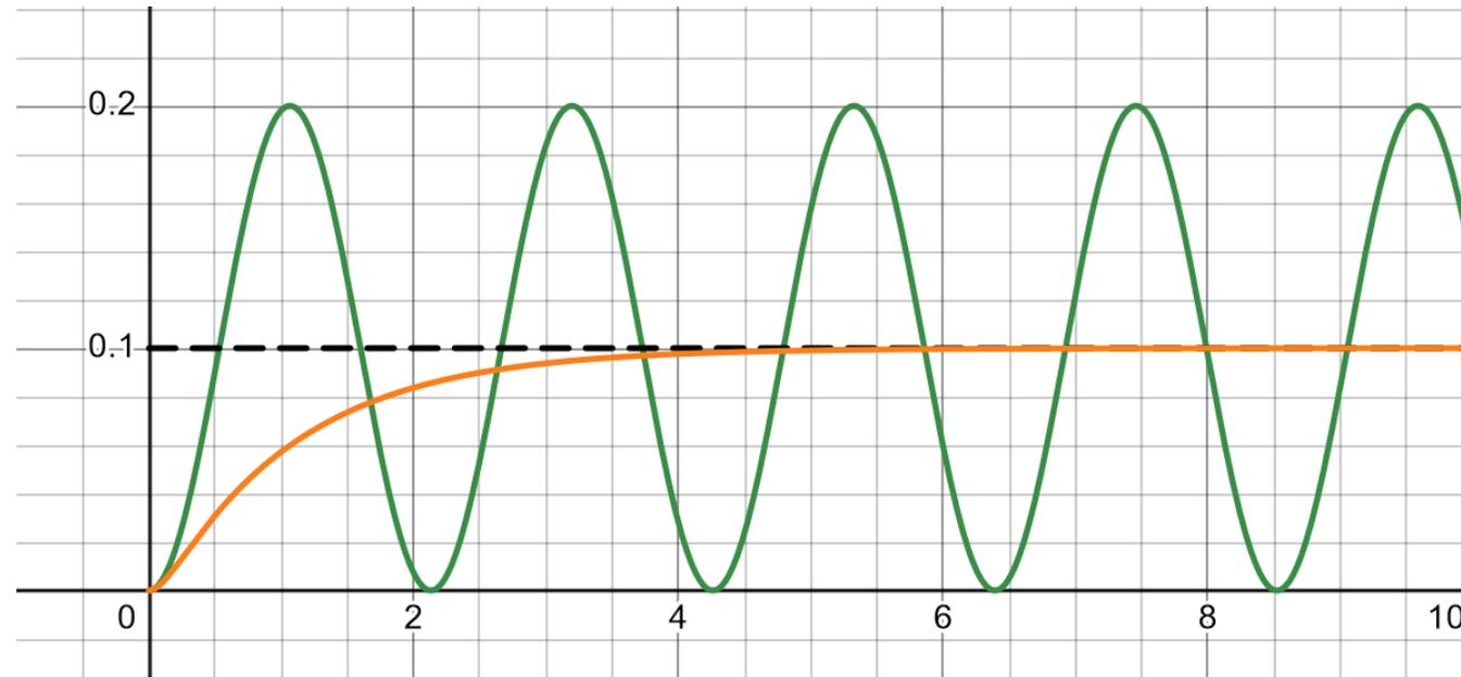
$$y(t) = r \left[ 1 - \left( \frac{1}{2} - \frac{k_d}{2\sqrt{k_d^2 - 4k_p m}} \right) \exp \left( \frac{-k_d - \sqrt{k_d^2 - 4k_p m}}{2m} t \right) - \left( \frac{1}{2} + \frac{k_d}{2\sqrt{k_d^2 - 4k_p m}} \right) \exp \left( \frac{-k_d + \sqrt{k_d^2 - 4k_p m}}{2m} t \right) \right]$$
