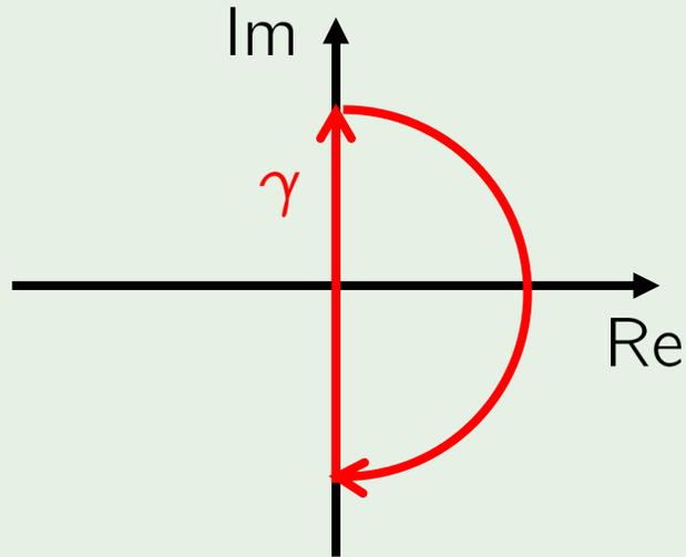
$$\begin{aligned} & \# \text{zeros of } 1 + L \text{ in } \mathbb{C}_{>} \\ &= (\text{winding number of } L(\gamma) \text{ about } -1) \\ & \quad + (\# \text{poles of } L \text{ in } \mathbb{C}_{>}) \end{aligned}$$
